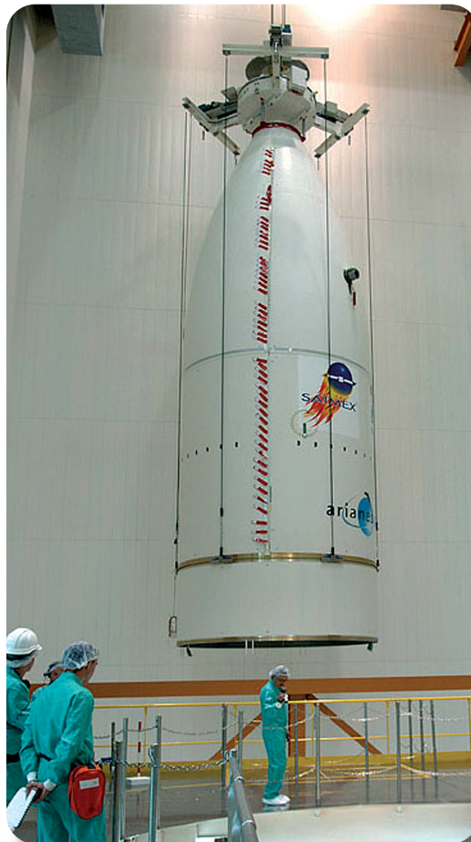
Cradle to lift and place payload fairing of an Ariane rocket
